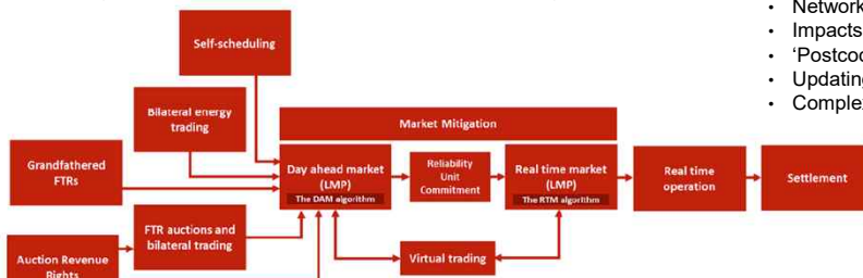
[Ref: Gill et al 2023 Exploring market change in the GB electricity system : the potential impact of Locational Marginal Pricing] Figure 8: Key elements of a typical LMP market [Ref: Tam & Walker 2023 Electricity Market Reform PN-694.]
