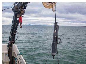
Water sampling with Niskin bottles using crane and winch
